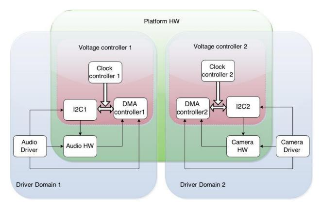
Figure 3. Complete hardware distribution between driver domains
